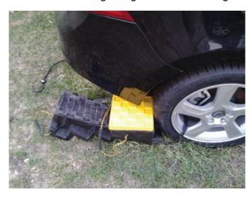
(2) The user positions the Cog Step as needed, with the cog wedge in close proximity to where it is needed to effect stabilization. As rescuers unweight the side of the vehicle, as they would to place a standard step chock, they introduce the Cog Step in much the same way. (*Photo by author.*)
