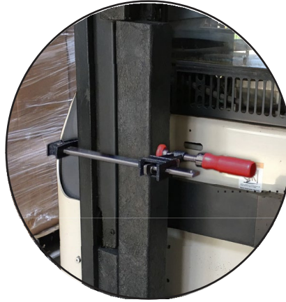
Example of mast support using both the FSS-4x4X22 and FSS-4x4x48 inner rail channel blocks.
