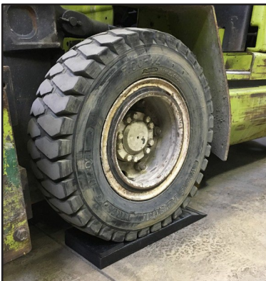
Example of a forklift on a Mfg. Part#: RZ-17-1-10 Stockpicker Rizer. DANGER: When driving on to the rizer, do so very slowly.
