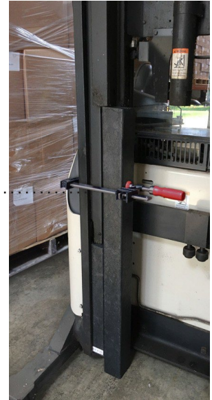
Example of mast support using both the FSS-4x4X22 and FSS-4x4x48 inner rail channel blocks.
