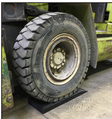
Example of a forklift on a Mfg. Part#: RZ-17-1-10 Stockpicker Rizer. DANGER: When driving on to the rizer, do so slowly.
