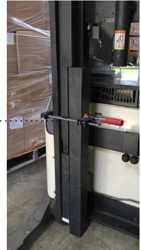
Example of mast support using both the 4" x 4" x 22" and 4" x 4" x 48" Dura Stat channel blocks.
