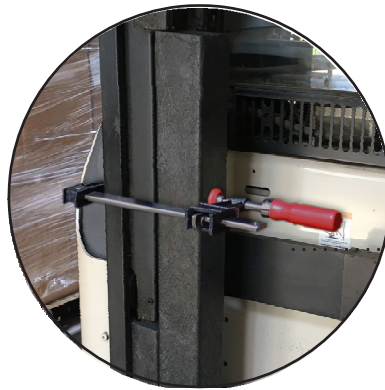
Example of mast support using both the 4" x 4" x 22" and 4" x 4" x 48" Dura Stat channel blocks.
