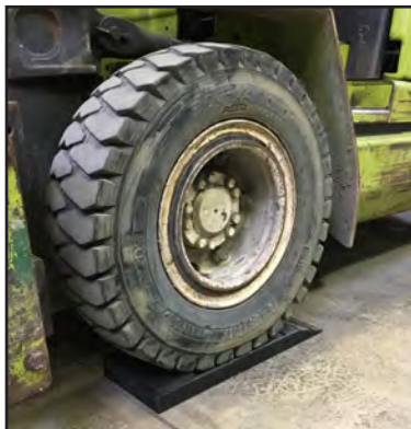
Example of a forklift on a stockpicker rizer. Note: When driving on to the rizer, do so slowly .
