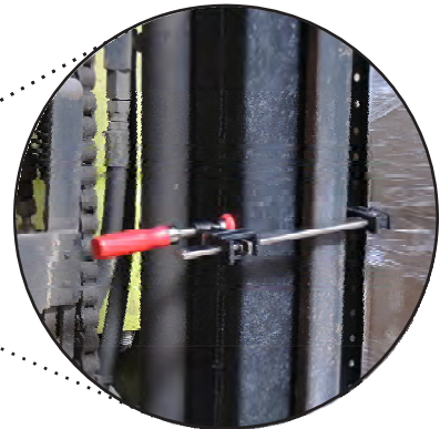
Example of a mast support using Mfg. Part# FSS-4x4x48 and Mfg. Part #FSS-Clamp.
