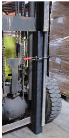
Example of mast support using both the 4" x 4" x 22" and 4" x 4" x 48" Dura Stat channel blocks.
