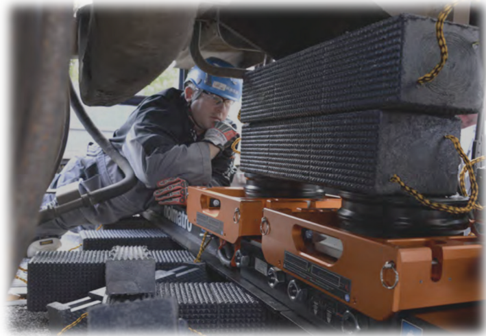
BLACK DIAMOND CRIB® (left and above) Mfg. Part # 67HDC-30 Working Load Limit: 71,600 kg/157,850 lbs. per block
