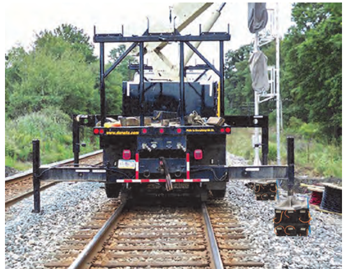
9 point box crib made with Prime Crib blocks Mfg. Part No. 67PC-24
