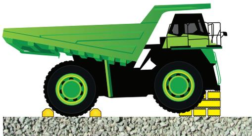
Use **dura crib** tools for **multiple layers** during repairs.
