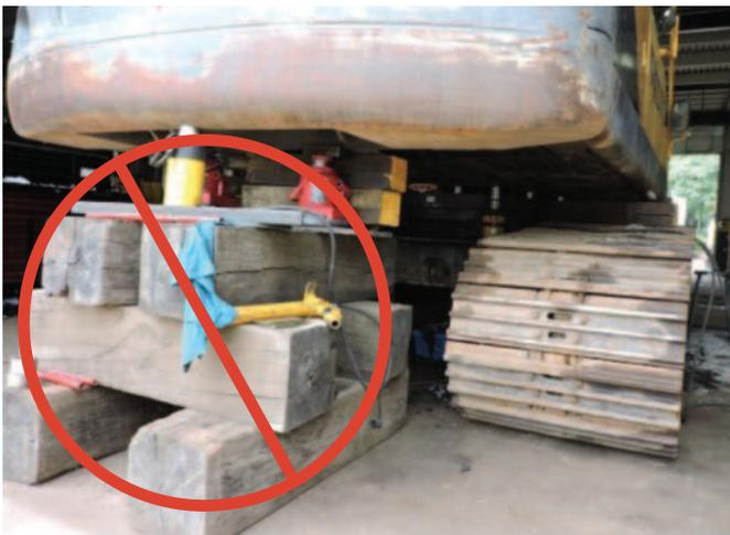
**UNSAFE REPAIR ENVIRONMENT USING WOOD CRIBBING**
