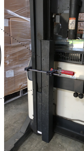
Example of mast support using both the 4" x 4" x 22" and 4" x 4" x 48" Dura Stat channel blocks.
