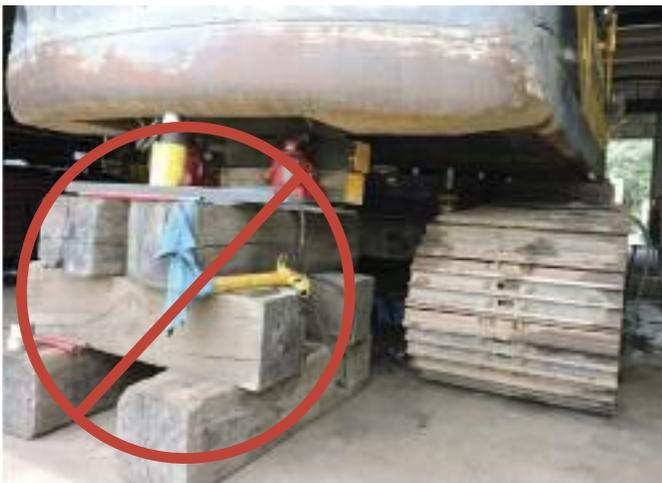
**UNSAFE REPAIR ENVIRONMENT USING WOOD CRIBBING**
